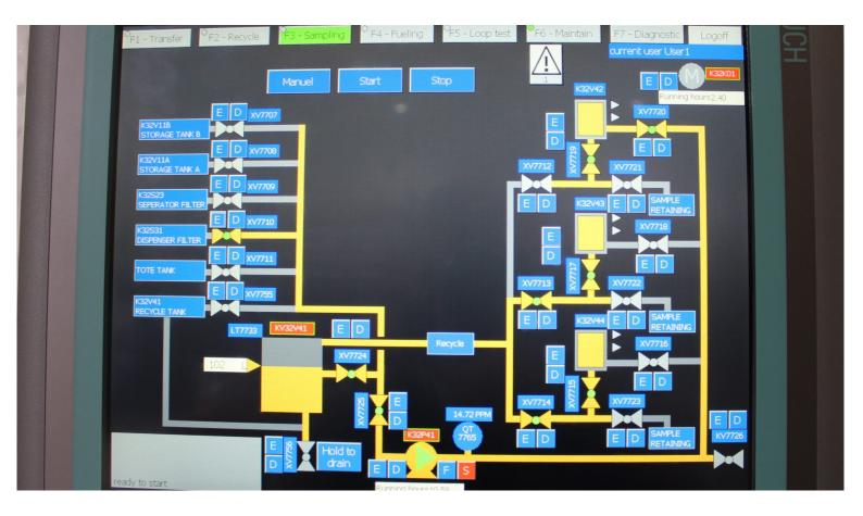
Imenco have standardized to Siemens programming tool TIA Portal Imenco have in-house expertise to meet any logical PLC programming request. We can provide services like SCD, functional and technical descriptions, logical control diagrams in addition to FAT procedures and in-house physical wiring and testing of the finished product.
