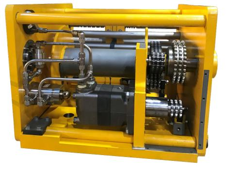
Intended for offshore subsea pulling operations by use of ROV The winch incorporates "API 17 D class 4 – vinger" fastened to the bottom plate for docking of the winch. The product is robust, compact and easily maintained. The winch drive is supplied by an orbital hydraulic motor & drive chain system.
