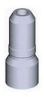
The internal profile will fit the Imenco GWA 22' and GWA 22'S Guidewire Anchors The Imenco Guidepost Tops – GPE profile has the standard Imenco GPE profile to enable installation of Guide Post Extension onto the top of the post. The Guidepost Tops – GPE profile is prepared for welding to 8in nom. pipe diameter (219mm OD).
