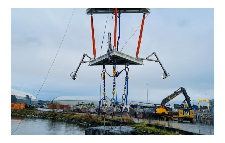
The Shackles can be remotely released by the operator
