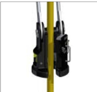
The Latch cable door is opened to insert tether cable into the latch.
