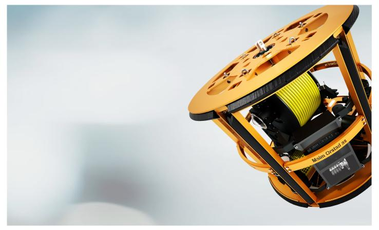
The Tether Management System makes the ROV more manoeuvrable and increases its range without moving the vessel or rig The purpose of the TMS is to lengthen and shorten the tether in order to minimize the effect of cable drag during underwater currents. The TMS is engaged to the ROV to make handling through the splash zone less hazardous during launch and recovery.
